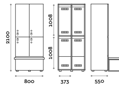
VANB45-23 Doppia colonna 4 ante per panca Double column 2-tiers locker, 4 doors, bench version
